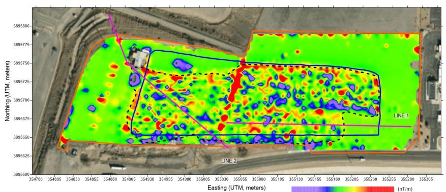
Figure 5. Contoured Magnetometry Results, Vertical Gradient (nT/m).
