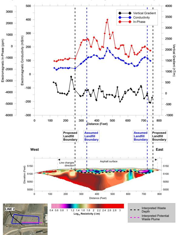
Figure 10. Line 2 Electrical Resistivity Comparison with EM & Mag Slices.
