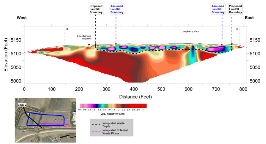
Figure 11. Line 2 Electrical Resistivity Profile.
