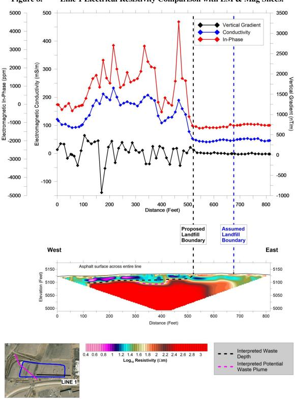
Figure 8. Line 1 Electrical Resistivity Comparison with EM & Mag Slices.
