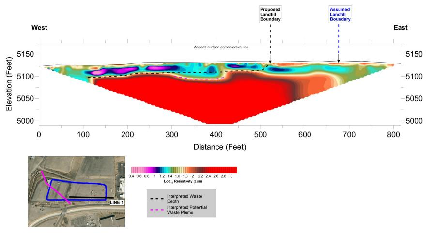
Figure 9. Line 1 Electrical Resistivity Profile.
