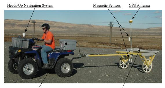
Magnetic Data Acquisition System and GPS Data Acquisition System
